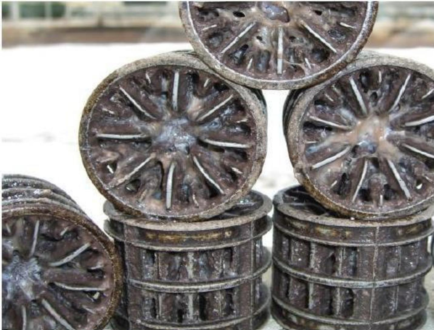
Figure 3: Blocked carrier (paper sewage water)
